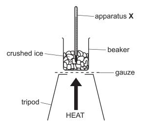
Every 2 minutes Oliver records the temperature using apparatus **X**.
